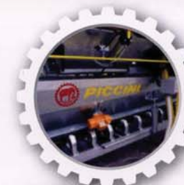
Aggregates weighing and extraction unit. The weighing hopper is entirely hot-galvanized and is composed by tanks with high capacity for a perfect filling and a rapid extraction of the product.
