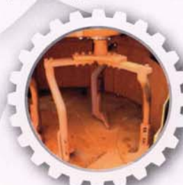
Planetary pan mixer, an absolute perfect mixing for any type of concrete, with rotating and satellites.
