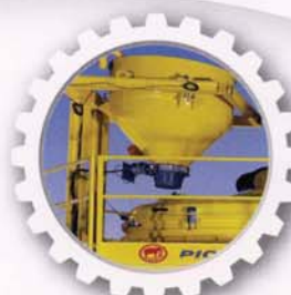
Cement doser with loading cells, vibrator in order to speed up the discharge, throttle valve controlled by double effect pneumatic actuator.
