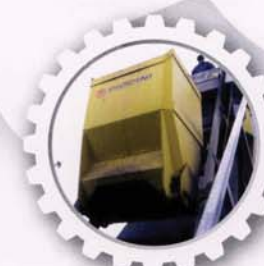
Aggregates loading skip towed by double winch with double steel rope. Double standard traverse speed.
